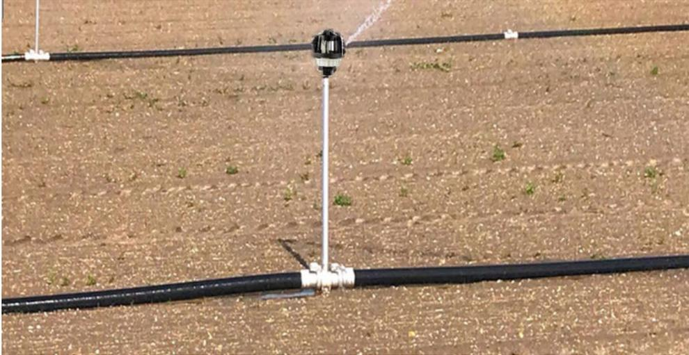
T M-H coupling (DN50-DN63) made of aluminium or PE.
